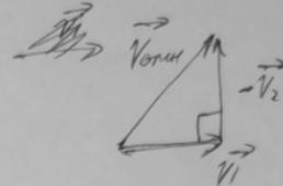
П.к.  $\vec{V}_1 \perp \vec{V}_2, V_{отн} = \sqrt{V_1^2 + V_2^2}$ .
