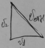
$$v_{отн}^2 = v_1^2 + v_2^2$$
