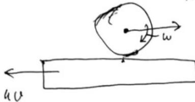
$M = M_{\text{кр}} - \mu mg R_{\text{ноб}} = \frac{1}{2} m R^2 \epsilon$
