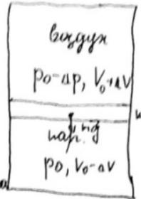
$(p_0 - \Delta p)(V_0 + \Delta V) = \nu_0 R T = p_0 V_0$
