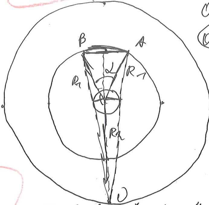
$$OB^2 = R_1^2 + R_2^2 + 2R_1R_2 \cos(\pi - \frac{\alpha}{2})$$
