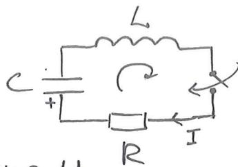
$$L \left. \frac{dI}{dt} \right|_{I_{\max}} = 0 \rightarrow U = I_{\max} R \rightarrow \underline{I_{\max} = \frac{U}{R}}$$
