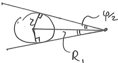
$$\sin \frac{\varphi}{2} = \frac{z}{R_1} = 0,1 \rightarrow \varphi \text{ - мал}$$
