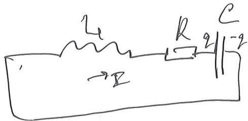
$$I = \dot{q} \quad \left| \begin{array}{l} 2x \cdot \omega = -\frac{R}{4\pi f C} \\ x = -\frac{R}{2L} \end{array} \right.$$
