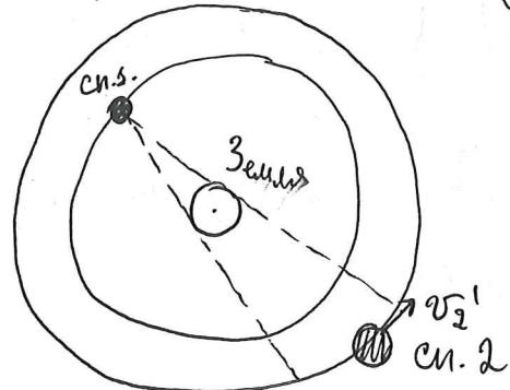
$v'_2 = \left| R_2 \cdot \left( \frac{v_2}{R_2} - \frac{v_1}{R_1} \right) \right|$
