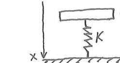
$$\begin{cases} x(t) = x_m \cdot \sin(\omega t + \varphi_0) \\ y(t) = \omega x_m \cdot \cos(\omega t + \varphi_0) \\ \text{ нач. усл. } x(0) = x_0 \\ y(0) = \dot{y}_0 \end{cases}$$
