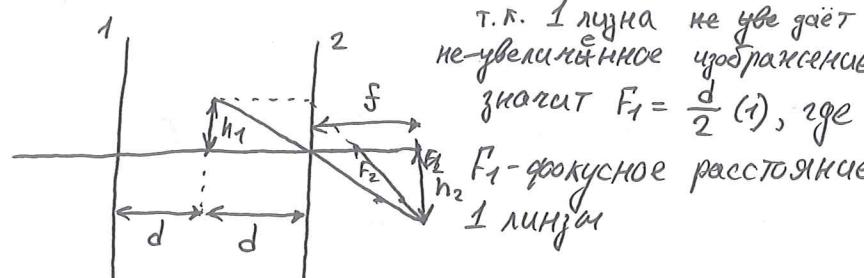
$$\Gamma = \frac{h_2}{h_1} = \frac{f}{d} \Rightarrow f = d \cdot \Gamma \quad (2)$$
