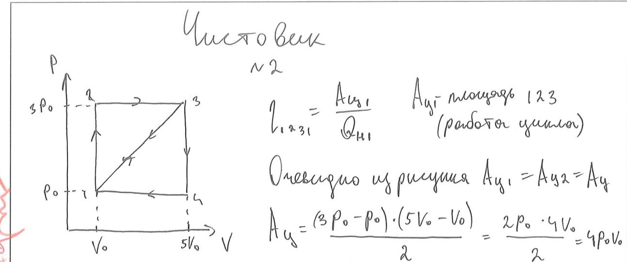
$$Q_{h1} = Q_{12} + Q_{23}; \quad Q_{12} = \frac{3}{2} \nu R \Delta T = \frac{3}{2} (3P_0 V_0 - P_0 V_0) = 3P_0 V_0$$
