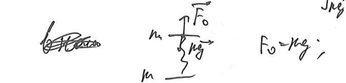
$$\text{Аналогия: } F_1 = 2mg ; \quad Kx_1 = 2mg ; \quad K_1 = \frac{2mg}{x_1}$$
